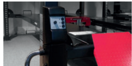
Control unit and power pack on rear left post
