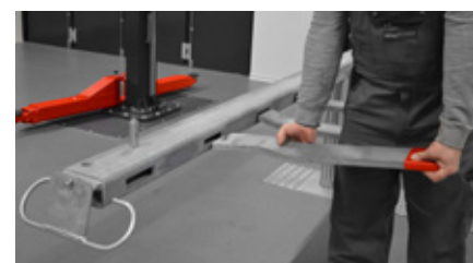
Fitting of lifting blades
