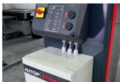
Pushbutton control and cabinet
