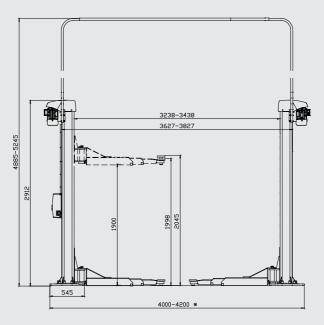
4000 mm: recommended for lifting transporter 4200 mm: recommended for universal lifting area, more focus on passenger cars
